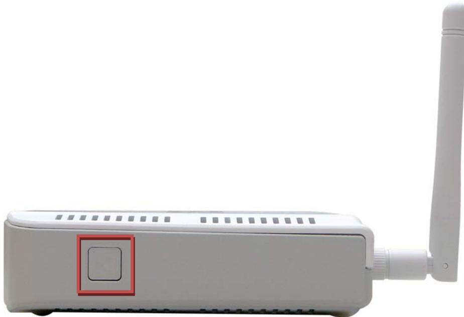
The WPS Push Button is located at the right side of the Router. Press the button to enable the WPS function. Refer to WPS section for more detail. The blue light blinks when searching for the connection. The blue light remains for 300 seconds when successfully connected.
